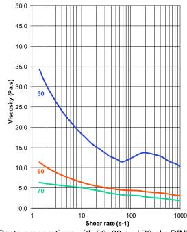
Paste preparations with 50, 60 and 70 phr DINP. Readings were made 1 h after preparation at 23 °C with rotational and capillary viscometers\*.
