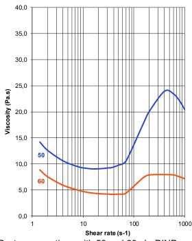
Paste preparations with 50 and 60 phr DINP. Readings were made 1 h after preparation at 23 °C with rotational and capillary viscometers\*.
