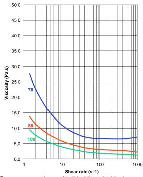
Paste preparations with 70, 85 and 100 phr DINP. Readings were made 1 h after preparation at 23°C with rotational and capillary viscometers\*.
